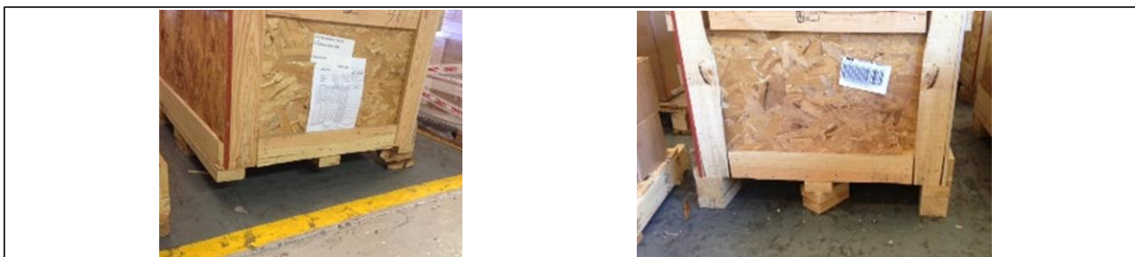
Picture 23 - Samples of Unacceptable Wooden Boxes Quality
