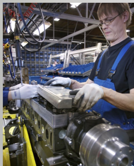
Technician fitting valve covers.
